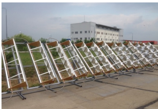
Figure 13. LS02 prototype – unit 1 (350x350 mm spot lenses, 32.5 mm focal length and copper tube)
