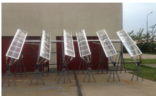
Figure 14. LS02 prototype – unit 2 (320x400 mm linear focus lenses, 62 mm focal length and vacuum tubes)
