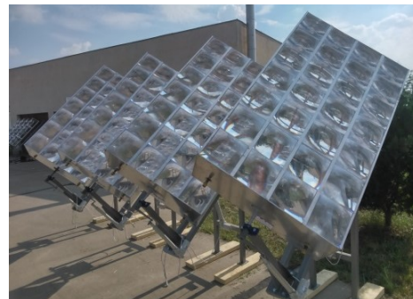
Figure 9. LS01 prototype – units 6-9 (250x250 mm spot focus lenses, 22.5 mm focal length)
