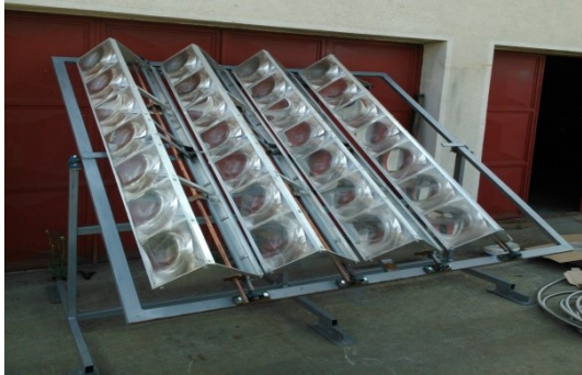
Figure 12. LS01 prototype – unit 20 (lenses with spot focus of 250x250 mm, focal length of 22.5 mm)
