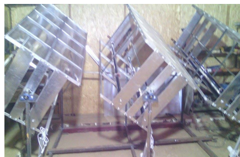
Figure 10. LS01 prototype – units 16-18 (320 x 400 mm linear focus lenses, 62 mm focal length and vacuum tubes)
