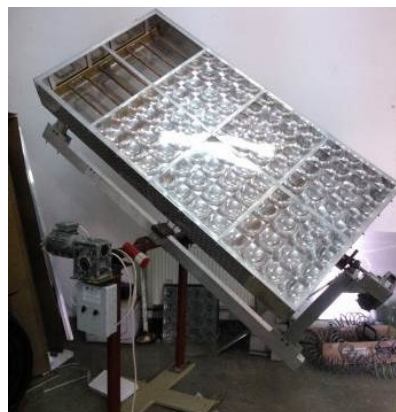
Figure 11. LS01 prototype – unit 19 (120x120 mm spot focus lenses, 120 mm focal length and driven by gear motors)
